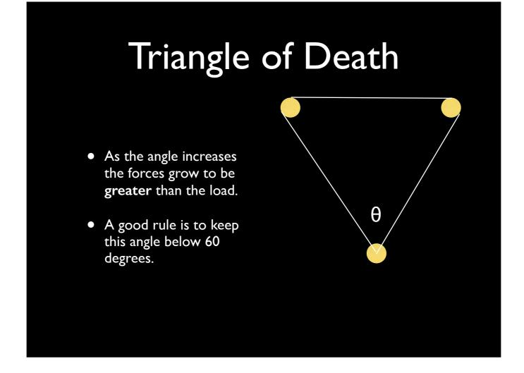
Using two points to rig form can spread the load out and make it safer. But done wrong it can actually make things more dangerous.
