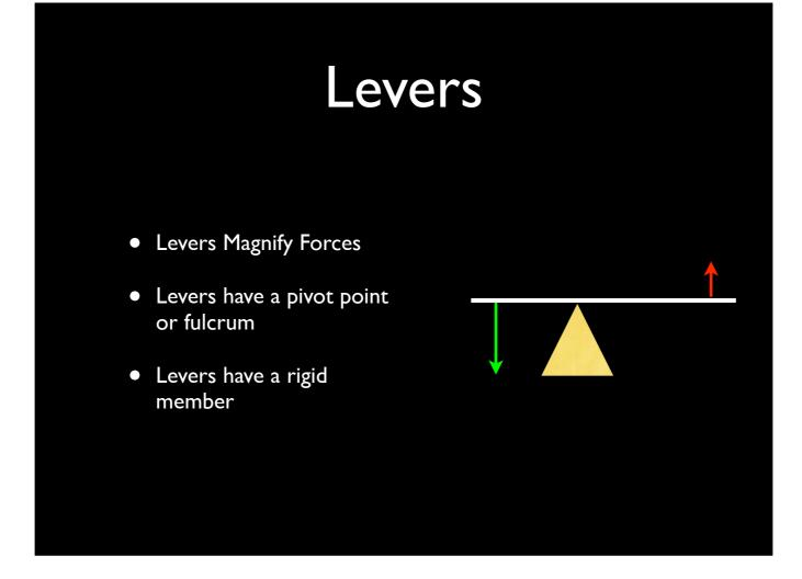
With levers the difference between the pivot point or fulcrum and the two forces determines how much force is needed on each end. A short lever has to use more force that a long one. But a long on has to travel farther to do the same amount of work.
