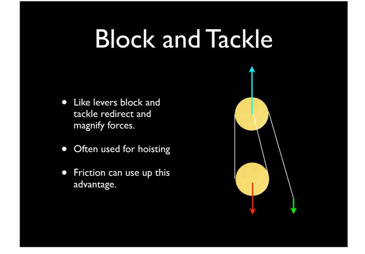
You can use an expensive block and tackle with ball bearings and rollers or you can simply run rope between two loops or carabiners to make a block and tackle. In the former you can assume almost no friction. When using the bight of your rope or a ring and carabiner friction will also reduce your advantage. Too many wraps and the friction will catch up and negate any advantage you gain.
